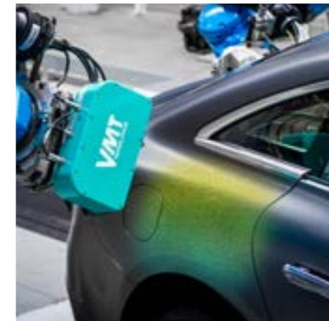
VMT™ OSC uses a shape-based measuring method for optical three-dimensional position determination. Instead of edges, holes or other concise object features, the geometric outer contour of a component or workpiece is used wholly or partially in order to determine its position or location and orientation.
