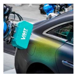
VMT OSC uses a shape-based measuring method for optical three-dimensional position determination. Instead of edges, holes or other concise object features, the geometric outer contour of a component or workpiece is used wholly or partially in order to determine its position or location and orientation.
