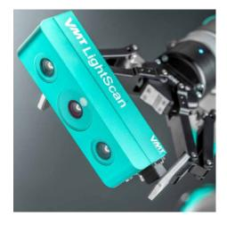
VMT OSC uses state-of-the-art 3D sensors for shape-based 3D measurement of the position and orientation of objects. Based on the stereo matching principle, the component is detected by two image sensors to calculate, for example, the 3D position of each individual pixel, regardless of its color, and in a manner that is resistant to extraneous light influences.
